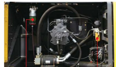
Fuel prefilter (with water separator) Pilot filter
